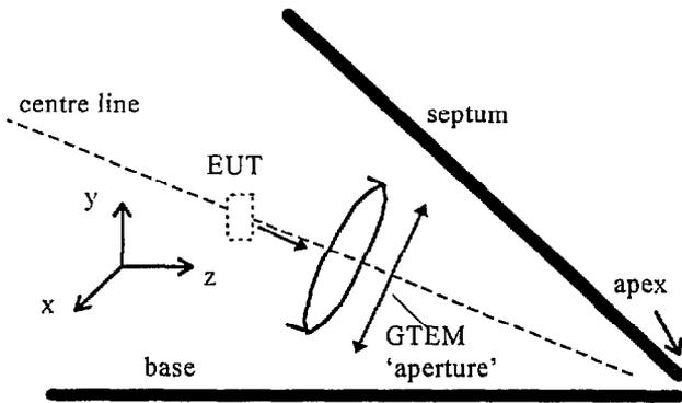
Figure 3. EUT measured in a GTEM
