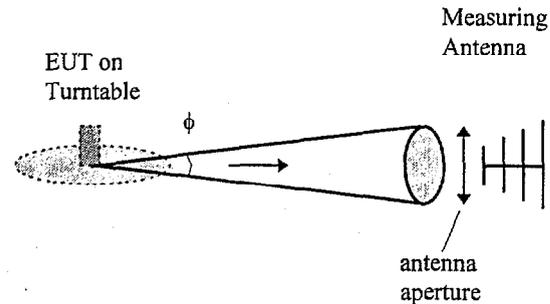
Figure 2. EUT measured in a Fully Anechoic Room
