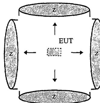
Figure 5. EUT measured with 4 Face Algorithm (Top View for Vertical Polarization)
