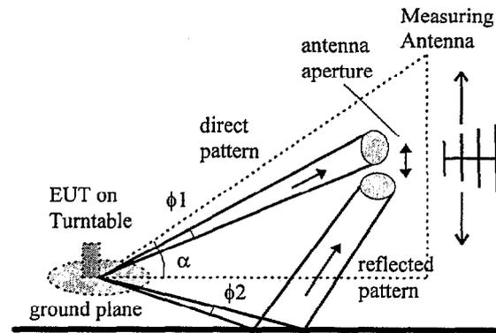
Figure 1. EUT measured on an OATS
