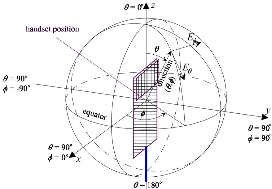
**Figure 60:** The dual-band patch antenna [59] in the standard spherical coordinate system [3, p. 16], as used in measurements/simulations. The patch points towards  $\phi = 90^\circ$ , the cable towards  $\theta = 180^\circ$ .
