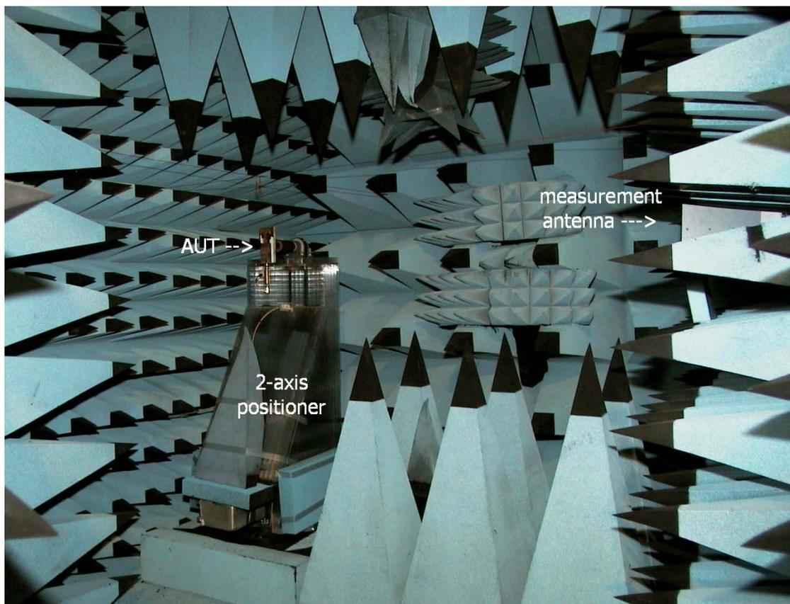
**Figure 26:** Small anechoic chamber at IDC, one side panel is open; we are looking at the opposite sidewall with 900 mm thick absorbers. Also ceiling and floor are lined with 900 mm long absorbers, other walls with 450 mm long RF absorbers. One antenna (wideband horn antenna, on the right) is fixed, acts as measurement or probe antenna, the AUT (left) is rotated about two axes, and its movements are computer controlled.
