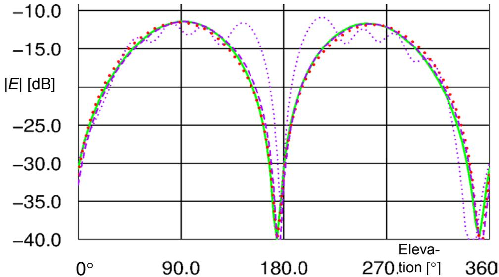
**Figure 57:** The H-plane radiation pattern at 1 GHz. Balun 1 is indicated by large dots, Balun 2 by a dashed line, the reference case without any cable attached is denoted by a solid line, and the far-field pattern with a 500 mm long cable attached and no balun is marked with smaller dots.
