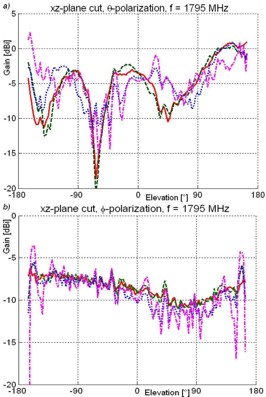
Figure 72. Comparison of  $xz$ -plane gain pattern cuts with four measured set-ups.  $f = 1795$  MHz. **M1: AUT + feed cable**  $\cdot - \cdot -$ , **M2: AUT + 3 ferrites**  $\cdot \cdot \cdot$ , **M3: AUT + balun**  $- -$ , **M4: AUT + balun and ferrites**  $-$ .
