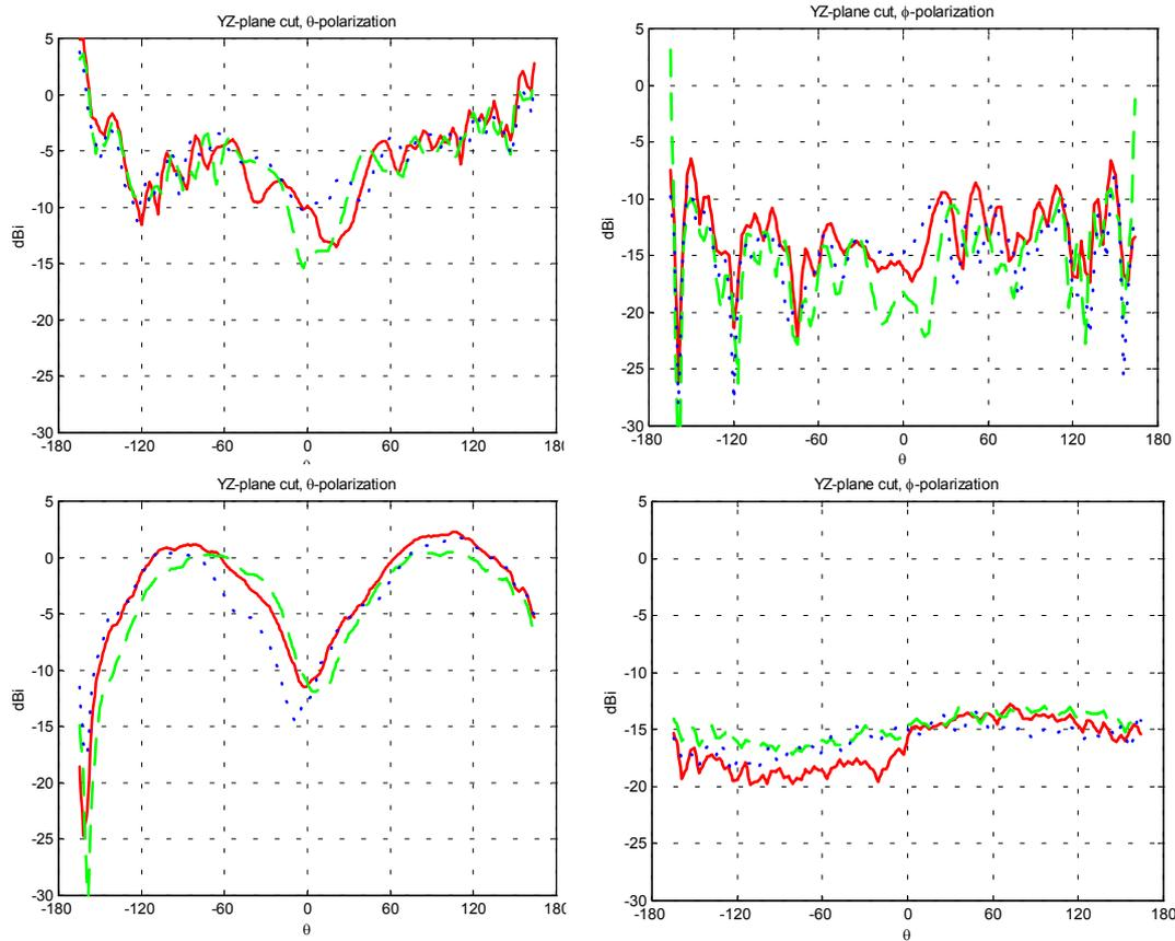
Figure 82. Illustrating the bandwidth of the balun at the GSM900 band. Gain pattern cuts at 880 MHz — — —, 920 MHz — — —, 960 MHz - - - -. *Top row: the worst set-up (M1: AUT + RF feed cable only). Bottom row: the best set-up (M4: AUT + balun + ferrites).*
