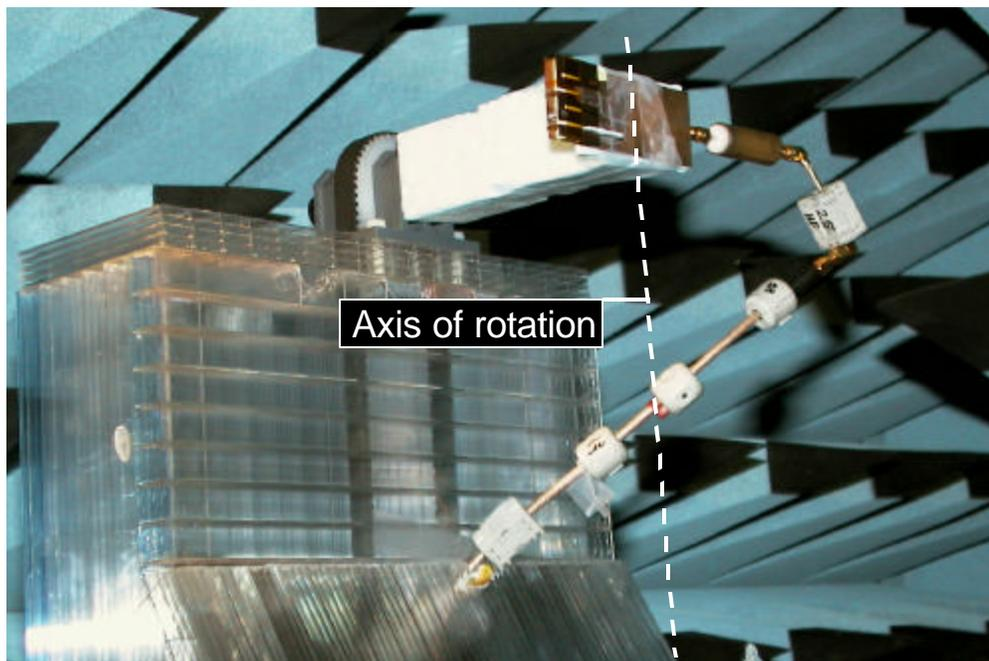
**Figure 33: Measurement set-up for the  $yz$ -plane pattern cut, i.e. the positioner was rotated around the vertical axis (dashed line), which translates to an elevation rotation for the AUT. The dual-band balun and five ferrites were placed along the RF cable.**
