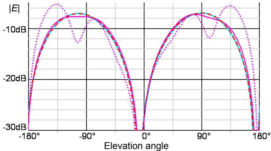
**Figure 54: Simulated  $yz$ -plane pattern at 920 MHz, short current dipole mounted on the corner of an 80 mm long handset, **isolated handset** — , **handset with cable** · · · , **with 1 balun** — , **2 baluns in a row** - - - .**
