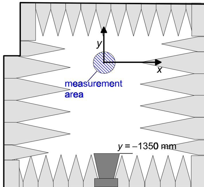
Figure 27: Measurement set-up for field homogeneity measurements in the quiet zone (i.e. the test volume) of the small anechoic chamber. Coordinate system as used in Figs. 28 – 31.
