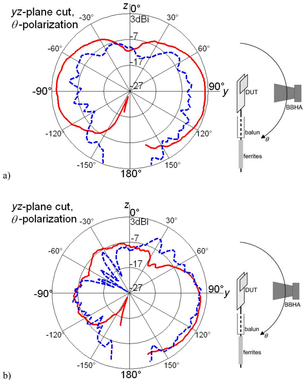
**Figure 75. Comparison of the yz-plane gain patterns for the worst set-up (M1, AUT + feed cable only) - - - and the best set-up (M4, AUT + balun + ferrites) —. The figure next to the plot visualizes how the AUT was oriented, a)  $f = 920$  MHz, b)  $f = 1795$  MHz.**
