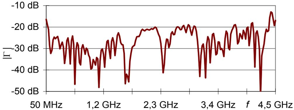
Figure 5: Magnitude of the reflection coefficient  $\Gamma$  of the termination section in the GTEM cell.
