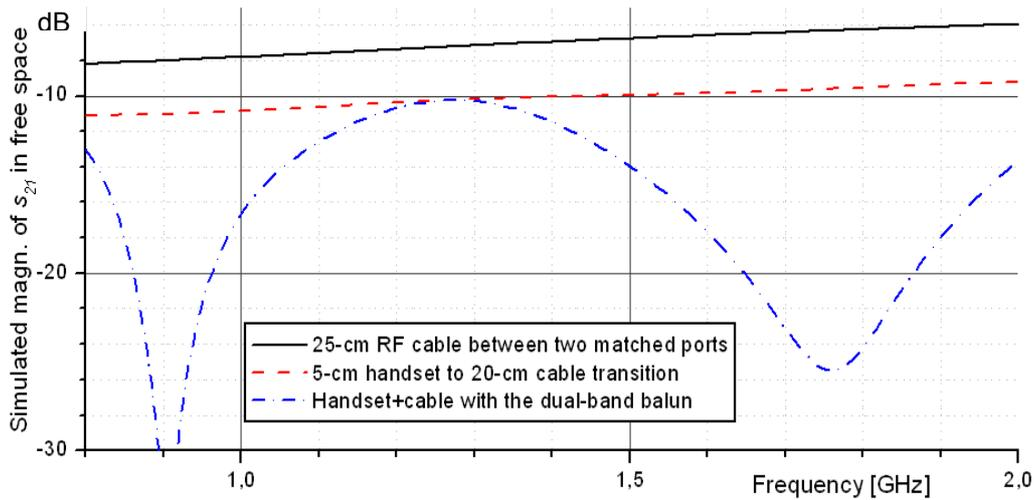
**Fig. 80:** Simulated  $|S_{21}|$  between two matched simulation ports 25 cm apart in free space, with (dash-dot) and without (dashed) balun on RF cable.
