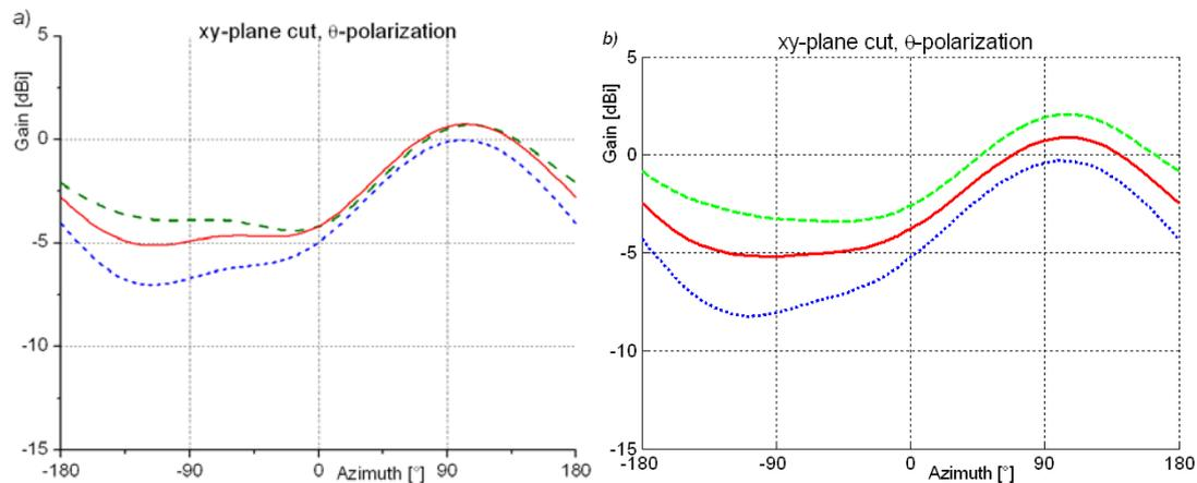
**Figure 85. Illustrating the bandwidth of the balun at the GSM1800 band,  $xy$ -plane, gain pattern cuts at 1715 MHz – – –, 1795 MHz —, 1875 MHz - - - -. a) simulated pattern with DUT alone, b) set-up M4) (DUT + balun + ferrites).**
