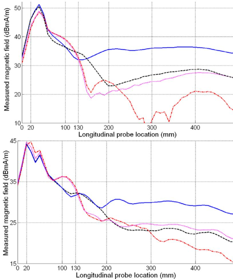
**Figure 78: The measured magnitude of the total  $H$ -field strength along the RF cable, 15 mm above ground plane (extends from 20 mm to 130 mm) and RF cable, at 920 MHz (top) and 1795 MHz (bottom). Cable only — (a) , with ferrites --- (b) , with balun — (c) , bal&ferr. - • - (d).**
