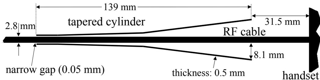
**Fig. 55: Cross-section of dual-band balun 1, indicating its location on the RF cable.**
