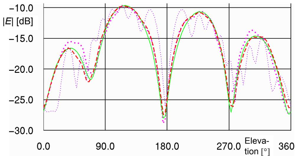
**Figure 58:** The H-plane radiation pattern at 2 GHz. Balun 1 is indicated by large dots, Balun 2 by a dashed line, the reference case without any cable attached is denoted by a solid line, and the far-field pattern with a 500 mm long cable attached and no balun is marked with smaller dots.
