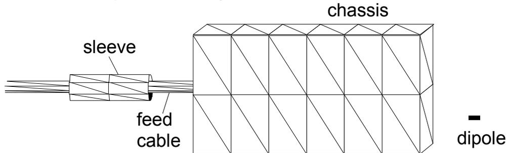
**Figure 51: Principle representation of the triangular mesh for the handset model simulated at 1 GHz. The actual mesh consists of 360 triangles. The cable continues to the left to a length of  $m_0 = 600$  mm.**
