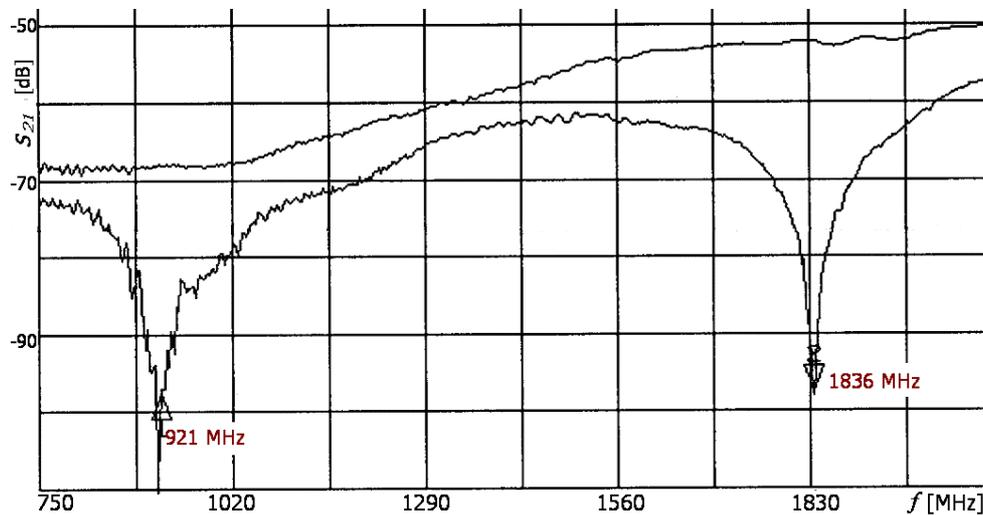
**Fig. 81:** Measured  $|S_{21}|$  between two capacitive field probes on the wall of the waveguide, with balun (lower) and without (upper) balun on centred RF cable inside a 52 mm × 72 mm rectangular waveguide (Fig. 79). The two resonance frequencies are 921 MHz and 1836 MHz.
