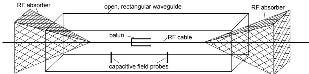
**Fig. 79: Principle measurement set-up for determining the filter characteristics of the balun inside a waveguide below cut-off.**
