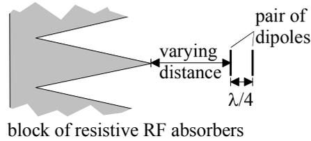
**Figure 19: Simulation set-up similar to the one for transmission measurements with a pair of dipole antennas positioned close to resistive absorbers.**
