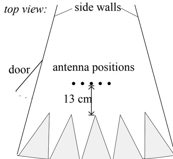
Figure 11: Measurement set-up when determining the field homogeneity inside the test volume of the GTEM cell.
