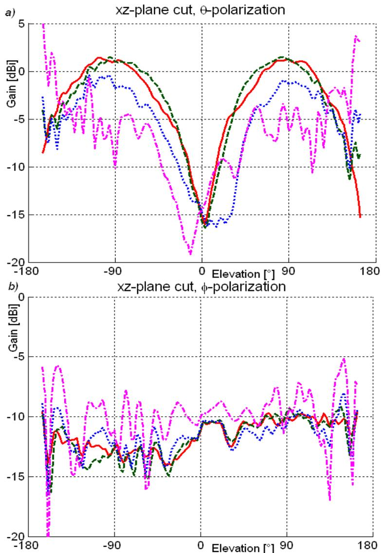
Figure 69. Comparison of  $xz$ -plane gain pattern cuts with four measured set-ups.  $f = 920$  MHz. M1: AUT + feed cable  $\cdot - \cdot -$ , M2: AUT + 3 ferrites  $\cdot \cdot \cdot$ , M3: AUT + balun  $- -$ , M4: AUT + balun and ferrites  $-$ .
