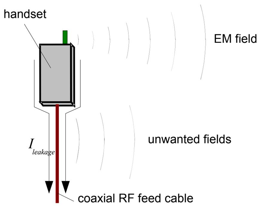
**Fig. 1: Illustration of influence of RF feed cable on radiated fields of AUT**
