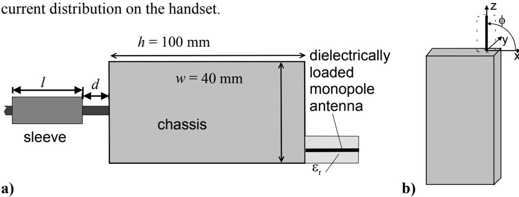
**Figure 47: a) Dimensions of simulated set-ups. The resonance frequency of the antenna is  $f_{res.} = 1 \text{ GHz}$ . The cable stub is attached to the bottom plane of the chassis. b) The coordinate system used in Figs. 48 and 49.**
