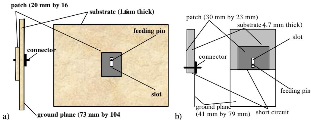
**Figure 4: The two experimental patch antennas used in the measurements, a) a  $\lambda/2$  patch antenna  $f_{res} = 3.76 \text{ GHz}$  and b) a  $\lambda/4$  patch antenna [46]  $f_{res} = 1.92 \text{ GHz}$ .**
