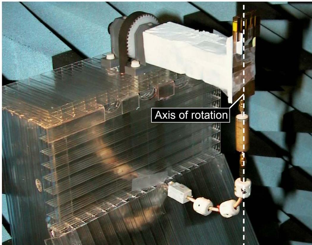
**Figure 34: Measurement set-up for the  $xy$ -plane pattern cut, i.e. the positioner was rotated around the vertical axis (dashed line), which translates into an azimuth rotation for the AUT. The quarter-wave dual-band balun between antenna and RF cable reduces the parasitic currents on the cable shield.**
