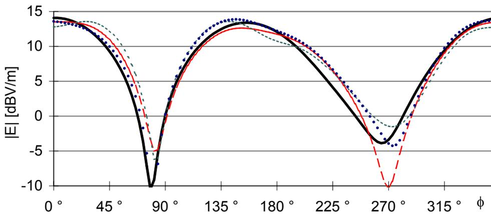
Figure 49: Simulated  $zy$ -plane radiation patterns at 1 GHz:  $|E|$  at 1 m distance, handset alone (solid), handset with 2.4 mm thick, 160 mm long cable plus cap 2 ( $l = 60$  mm,  $d = 15$  mm, dash-dot), cap 3 ( $l = 60$  mm,  $d = 20$  mm, dots), and cap 4 ( $l = 65$  mm,  $d = 10$  mm, dotted).
