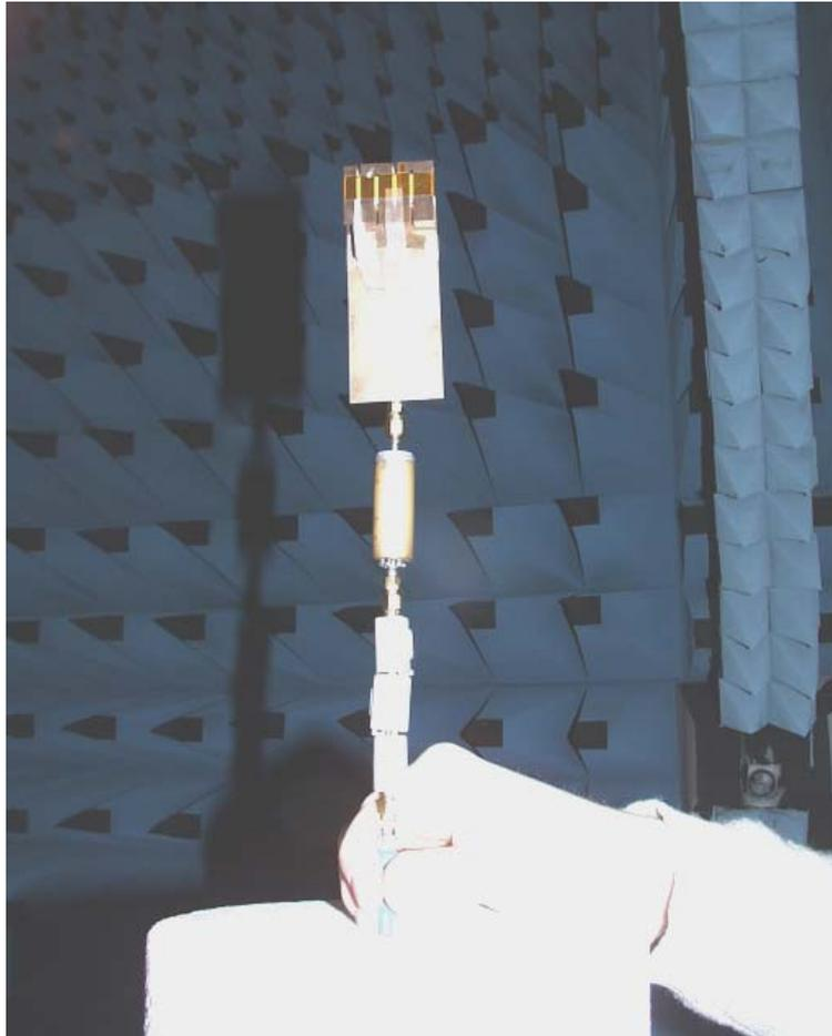
**Fig. 64. The AUT (top) with the dual-band balun and three ferrite beads (bottom).**
