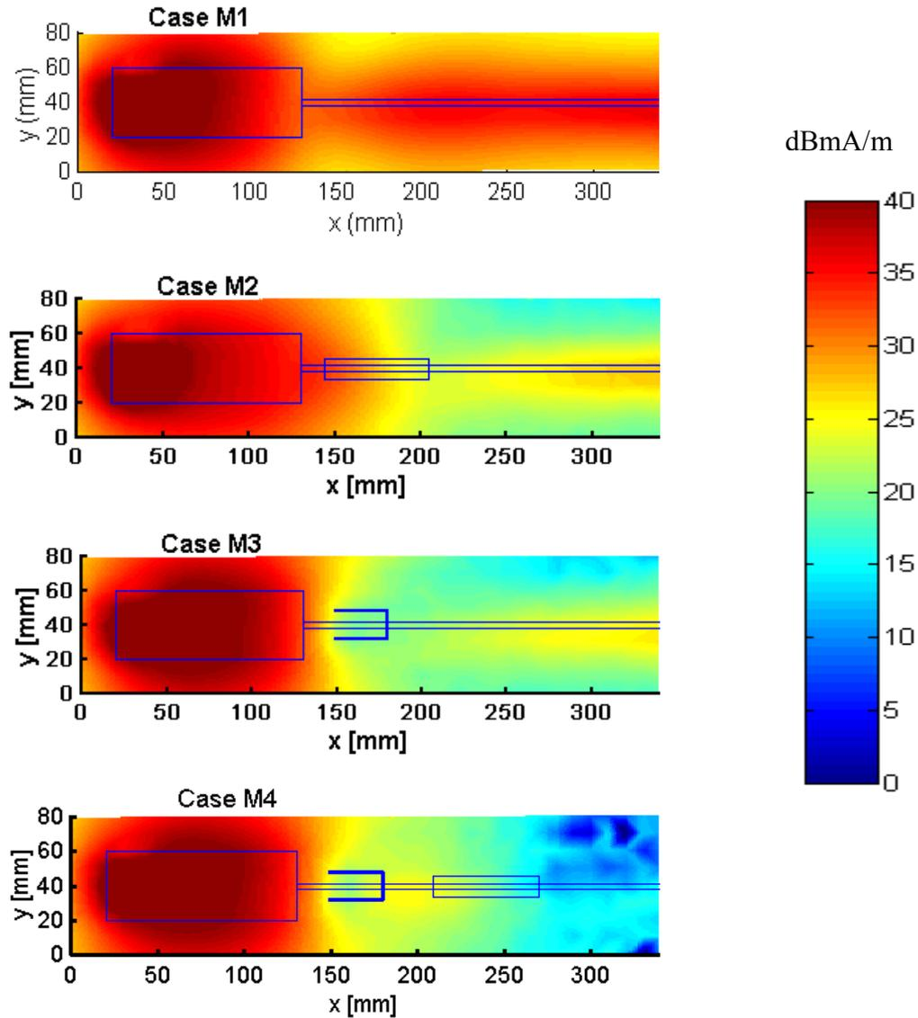
Figure 76: Measured magnitude of total H-field [dBmA/m] 15 mm above the ground plane at  $f = 920$  MHz, The ground plane (40 mm  $\times$  110 mm), the RF cable, and the location of the 3 ferrites (total length = 70 mm,  $\varnothing = 14$  mm) are adumbrated by thin lines, the balun (length = 44 mm,  $\varnothing = 16$  mm) by a thick line.
