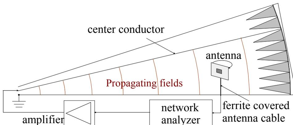
Figure 3: Antenna measurement set-up inside GTEM cell.
