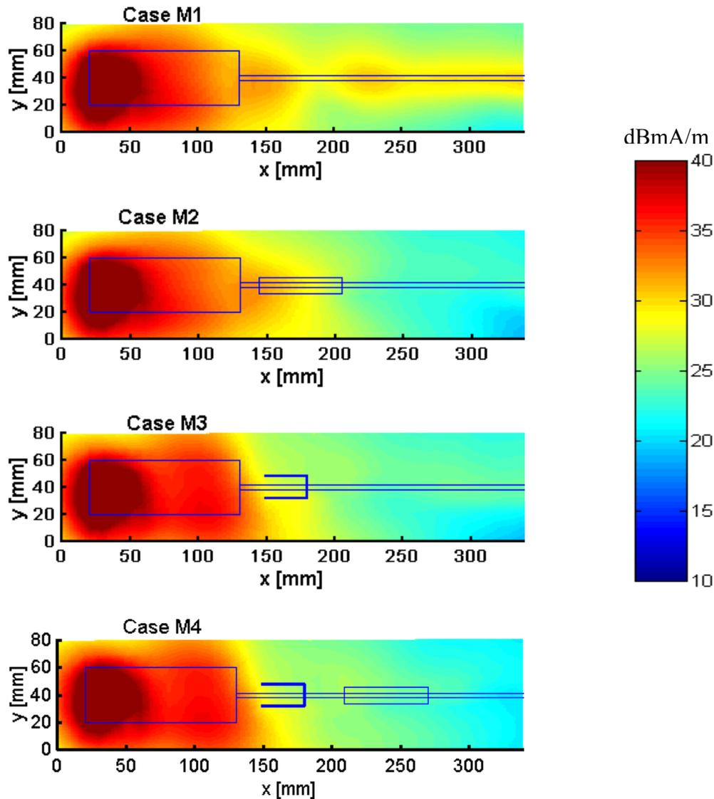
**Figure 77: Measured magnitude of total H-field [dBmA/m] 15 mm above the ground plane at  $f = 1795$  MHz, The ground plane ( $40 \text{ mm} \times 110 \text{ mm}$ ), the RF cable, and the location of the 3 ferrites (total length = 70 mm,  $\varnothing = 14 \text{ mm}$ ) are adumbrated by thin lines, the balun (length = 44 mm,  $\varnothing = 16 \text{ mm}$ ) by a thick line.**
