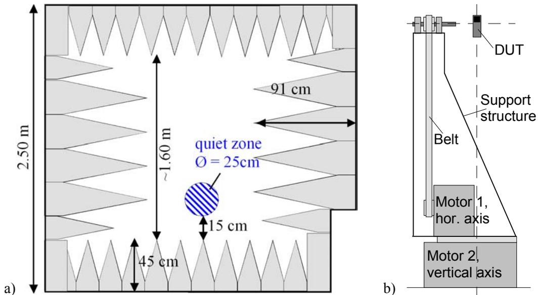
**Figure 25:** a) Design of small anechoic chamber at IDC, with 2.5 m long and 2.4 m high sidewalls. b) Automated positioning system with a vertical and a horizontal axis (dashed lines), the latter driven via a belt, DUT in the centre of rotation = centre of ‘quiet zone’.
