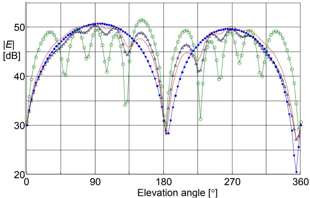
**Figure 52: Simulated electric field strength at 10 m distance from source. The solid line indicates the complex sum of the radiation patterns with five slightly different cable lengths, the reference case without any cable attached is denoted by dots, and the far-field pattern with a 600 mm long cable attached and no sleeve is marked with circles. Additionally, the radiation pattern based on the balun dimensions proposed in Section 5.1.1 and in [39] is shown with triangles.**
