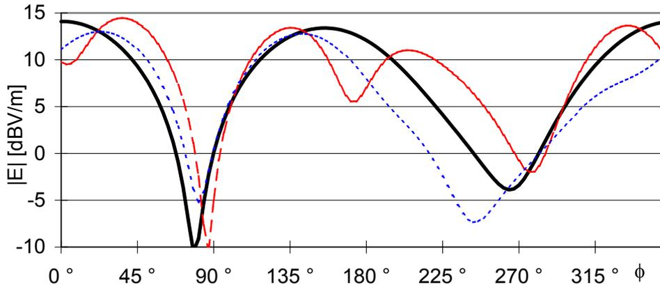
Figure 48: Simulated  $zy$ -plane radiation patterns at 1 GHz:  $|E|$  at 1 m distance, handset alone (solid), handset with 2.4 mm thick, 160 mm long cable (dashed), and a ferrite bead ( $l = 80$  mm,  $\varnothing = 20$  mm,  $\epsilon_r = 50-j5$ ,  $\mu_r = 50-j5$ ) attached to cable at  $d = 30$  mm (dotted).
