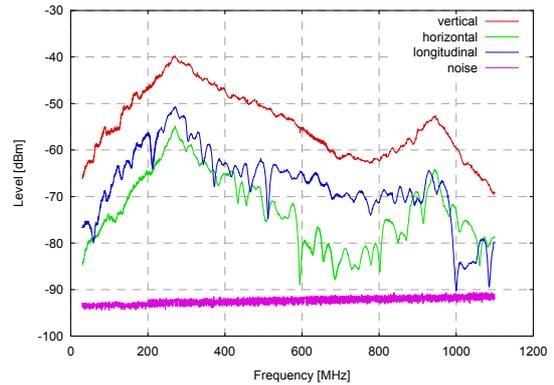
**Figure 15: Field components in a top corner of the nine-point grid**
