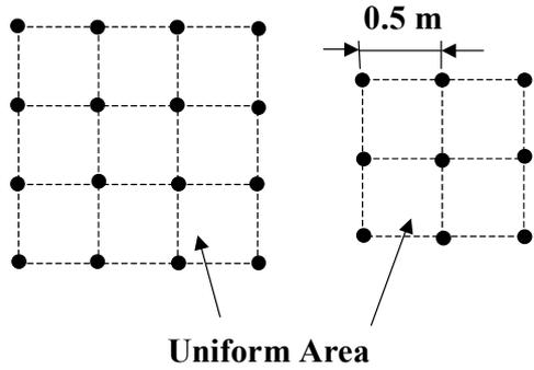
**Figure 12: The 16-point and the 9-point grid for field uniformity**
