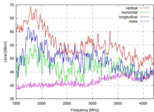
**Figure 16: Field components in a central point of the 16-point grid**
