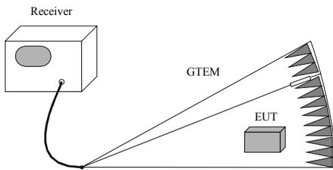
**Figure 2: Emission measurement setup**
