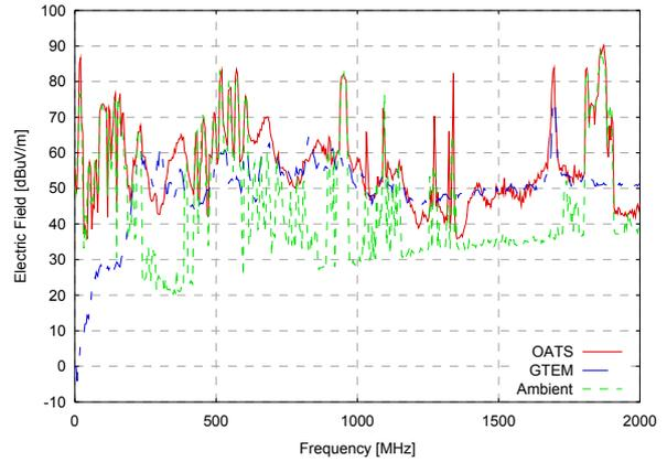
**Figure 7: GTEM-OATS Comparison for maximum radiation of REUTE in Slot and Gap Mode, 10 m**
