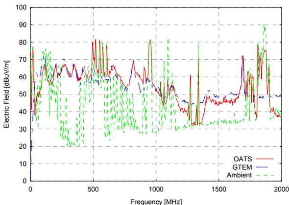
**Figure 11: GTEM-OATS Comparison for maximum radiation of REUTE with fixed cable, 10 m**
