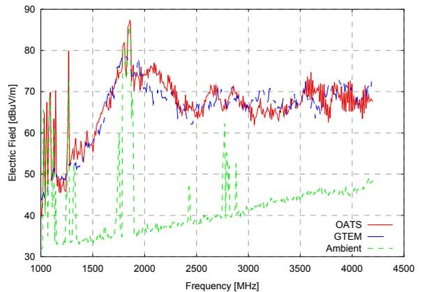
**Figure 9: GTEM-OATS Comparison for maximum radiation of REUTE in Slot Mode, 10 m**
