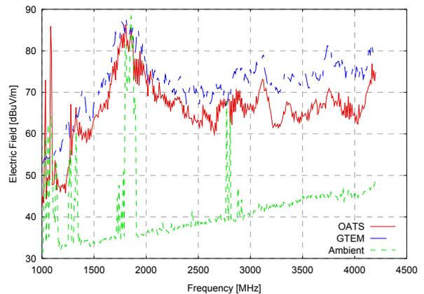
**Figure 8: GTEM-OATS Comparison for maximum radiation of REUTE in Gap Mode, 3 m**
