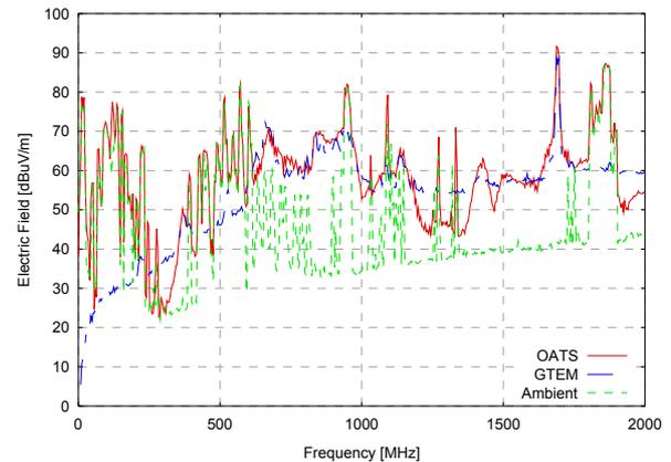
**Figure 4: GTEM-OATS Comparison for REUTE in Slot Mode, vertical polarisation, 3m**
