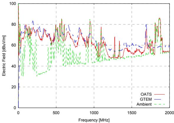
**Figure 10: GTEM-OATS Comparison for maximum radiation of REUTE with loose cable, 10 m**
