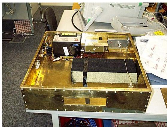
**Figure 1: Radiating EUT showing battery (top left), 7 GHz CNE (top centre), 2 GHz CNE (top right)**
