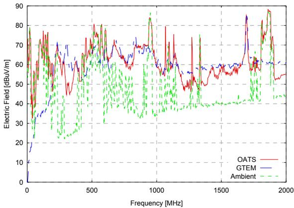
**Figure 6: GTEM-OATS Comparison for maximum radiation of REUTE in Slot and Gap Mode, 3 m**
