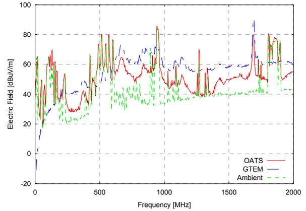
**Figure 3: GTEM-OATS Comparison for REUTE in Slot Mode, horizontal polarisation, 3 m**
