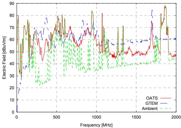
**Figure 5: GTEM-OATS Comparison for maximum radiation of REUTE in Gap Mode, 3 m**
